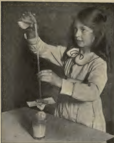
FIG. 151. Pouring the syrup into the "osmosis tube."
